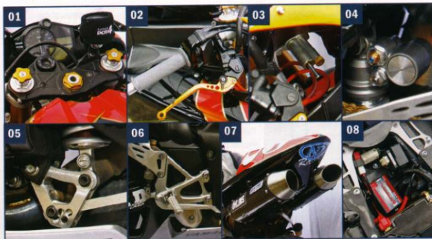
1. Valtor Moto preload adjusters. 2. CRG levers. 3. Ohlins steering damper. 5. Revvalved standard shock. 5. Roaring Toyz rear linkage. 6. Stock pegs. 7. GYTR exhaust. 8. Power Commander.
